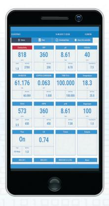
View your controllers readings and settings. Use detailed parameter graphs to track up to 5 years previous readings. Receive individual parameter alarms, via SMS and email.
