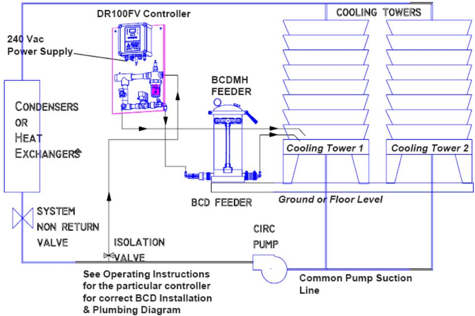
1. The pH and ORP controllers house sensitive electronics and preferably should be installed internally in the plant room, or if external should be installed in shade and protected from direct sunlight and temperature extremes.
