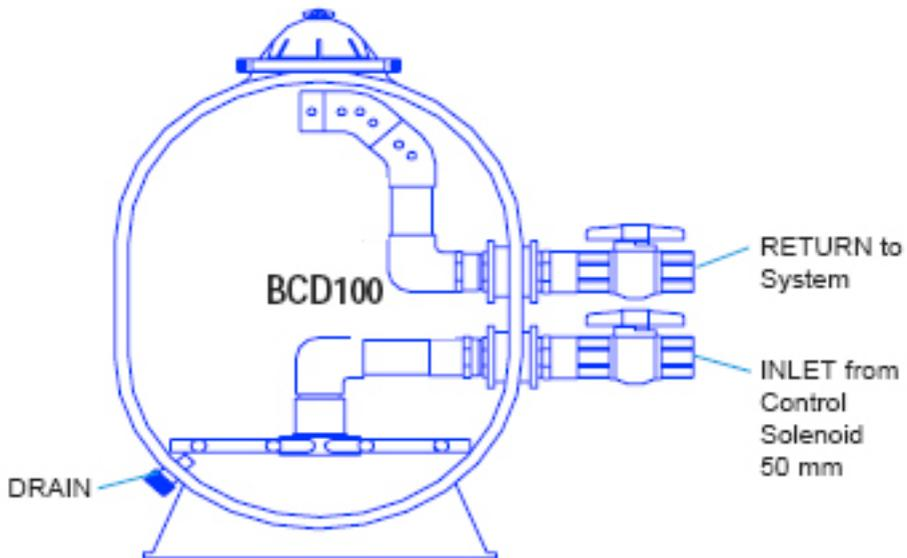
1. Attach the 50 mm valves supplied as shown in the diagram above.
