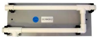
The **Aquarius Corrosion coupon exposure racks** are designed to retain the coupons in the laminar flow region and away from the turbulent flow areas around the Tee sections. The velocity across the coupons can be controlled via the isolation valves to represent flow conditions and velocities in heat exchangers.
