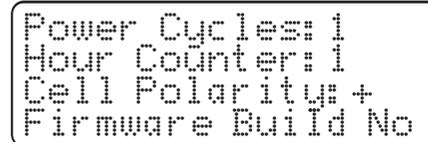
**POWER CYCLES** The number of times the Chlorinator has had power removed and applied.
