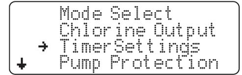
The TIMER SETTINGS can be programmed to turn the chlorinator ON or OFF in one hour segments over the course of a 24 hour day.
