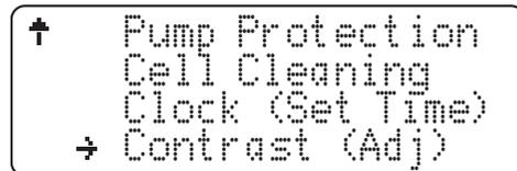
Use the [▲] button to increase the contrast level, and the [▼] button to decrease the contrast level.
