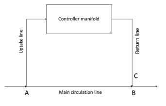
Manifolds with bowls for probes are more susceptive to pressure drop.
