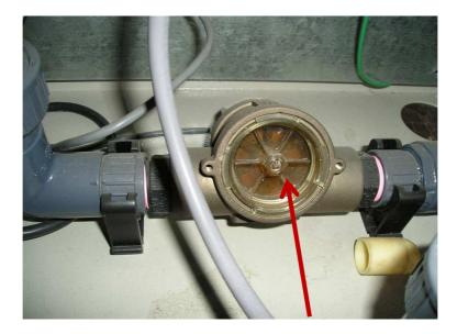
6. Using AquaReporter set the flow velocity mode to Auto and Change the velocity set points to different numbers (e.g., 0.5m/s, 1.5m/s and 2.5m/s) and watch the flow control valve each time. The Flow control valve should automatically rotate to different positions to set the velocity. If this has not happened, the Flow Meter is blocked and hasn't sent the correct signals to Flow control valve. Clean or replace the flow meter.
