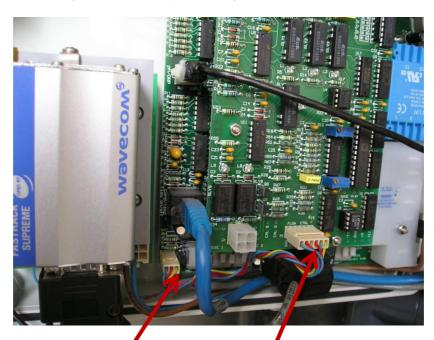
2. Check the following soldered wires have not snapped off.
