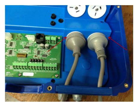
Wire the provided no volt output cables into the pumps as they are labelled for.
